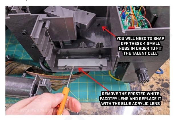
10. Install the new acrylic blue power cell lens. The lens is designed to be a direct fit without cutting the proton pack. Then reinstall the power cell cover.
