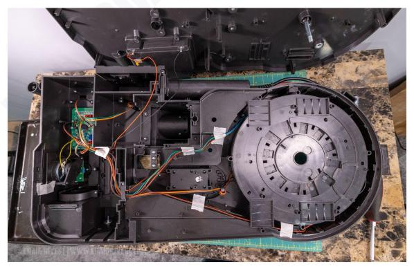
3. Disconnect the yellow BAT1 connector from the main board and set aside the back cover. You can coil this wire up and tape it to the back cover's inside if you wish. You won't be needing it anymore.
