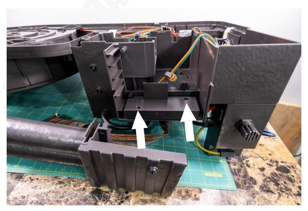
9. Use a small screwdriver and pop up the factory frosted white lens cover. You will also need to break off these 4 small nubs with pliers. This is where the Talentcell will be placed later.
