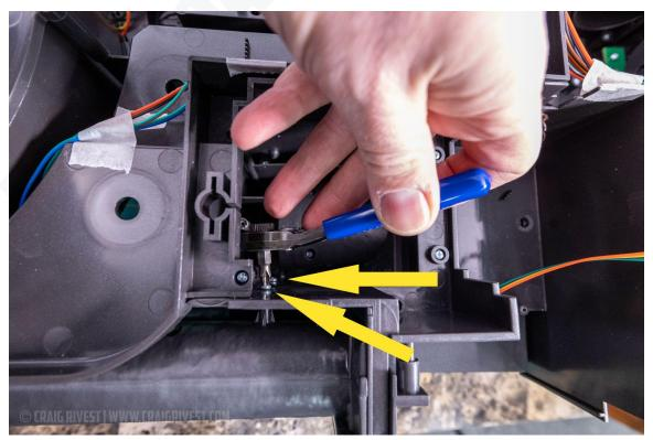
7. Remove two screws that hold the storage compartment door and pull the door out towards you. (Ignore the Talentcell in this photo, we'll install it later on).
