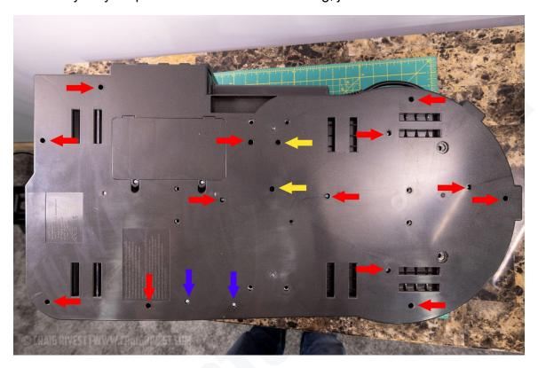
The back cover should now snap off, work slowly around the edges and lift straight up. Once the cover is off, be careful not to over extend the connected factory power wires. They go from the back cover to the BAT1 location on the main board.
