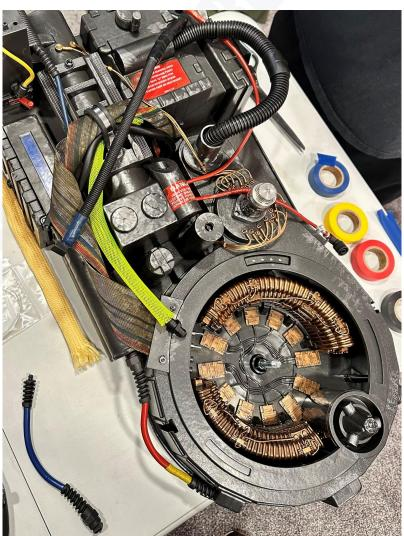
2. Remove the battery door and then the 17 back cover screws. The screws marked with blue are shorter, so keep track of those. The screws marked yellow hold the Filler and Beam line on (the two cylindrical tubes) in place on the front, so they may drop out or twist when unscrewing, just be mindful of that.
