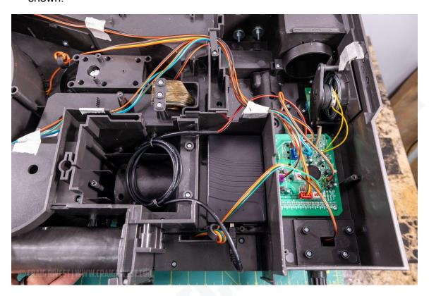
Install the JST to USB power cable as shown. You may be tempted to power everything on now to test. However, the pack will not power on until the cyclotron is properly installed. You can now reassemble the pack, watch for wires when reassembling.
